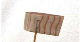
the back down to a point about 1/16" thick. Add fiberglass cloth to the sides of the rudder to make it more durable.
