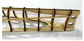
9. Cut out the centers of the ribs between the double keels. This will form the water channel for the pump.
