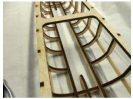
10. Using a plane and/or sanding block, blend the sub-deck with the ribs.
