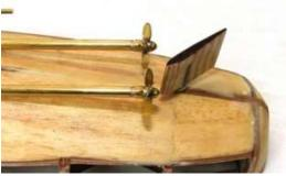
hull, making sure that the props are close to, but slightly ahead of the rudder. The rudder should move freely from side to side without hitting the props. Check that the stuffing shafts are fully through the ribs inside the hull and then glue in with epoxy, forming a small fillet around each shaft to ensure a water tight joint.
