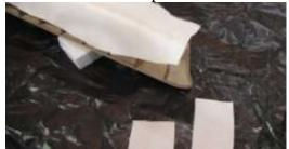
around these areas. Start by pouring a small bead of epoxy on the cloth along the center of the hull, and then use a brush or squeegee to spread it to the edges. Allow plenty of time for the epoxy to work through (wet) the fiberglass before adding more epoxy. Work on a small area at a time, and
